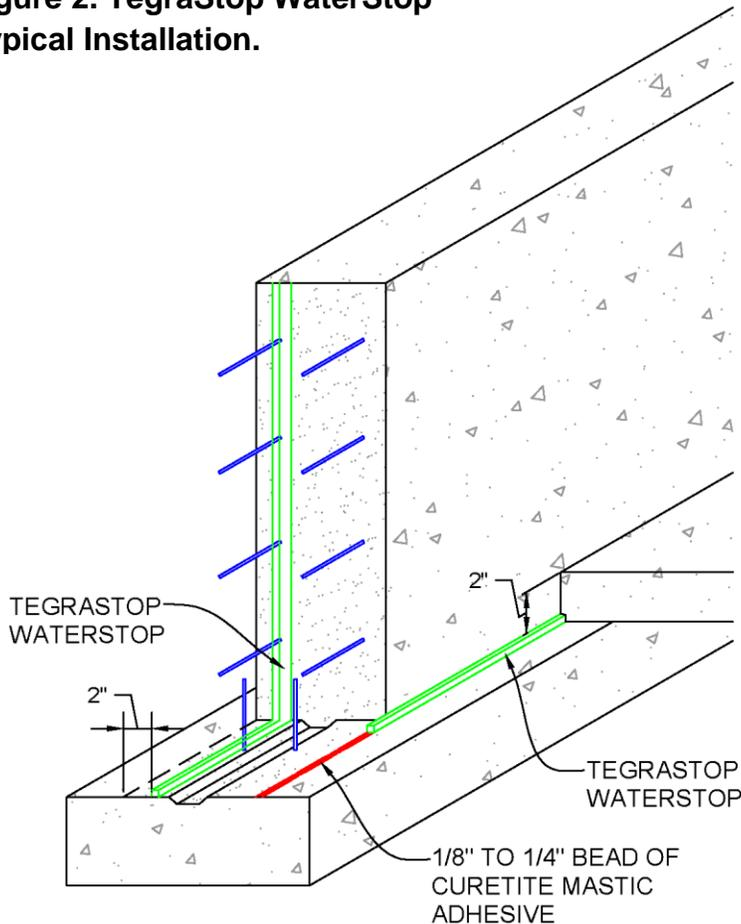
Use TegraStop™ WaterStop on vertical and horizontal construction joints with 2" of containment. CureTite™ Mastic Adhesive will fill voids in rough concrete and provides additional adhesion to the concrete while preventing water or concrete from seeping under the TegraStop WaterStop.
